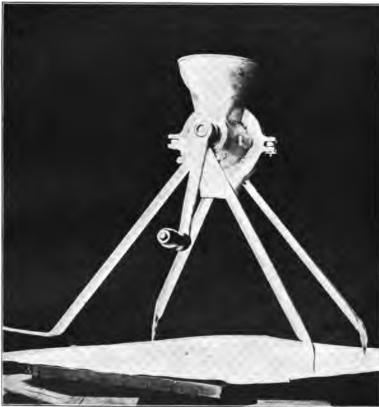
Figure 5.—COAL GRINDER SHOWING METHOD FOR ATTACHING LEGS.
